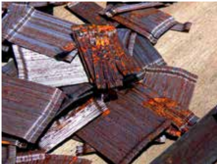
Corrosion of Steel Fibres
