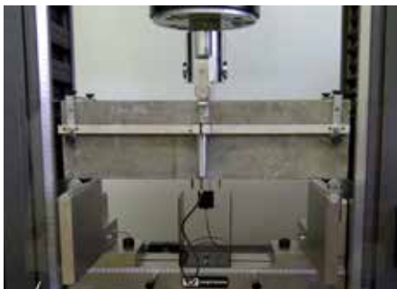
Image 1: EN 14651 Notched Beam Test
